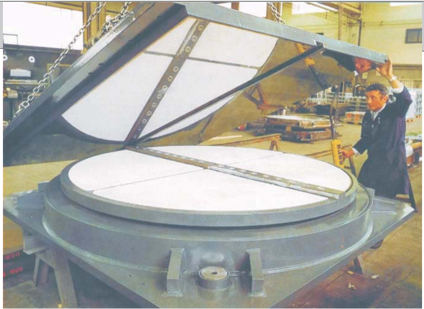
Detalji proizvodnje čeličnih delova Algapot ležišta uz upotrebu najmodernije tehnologije Manufacturing details of steel components of Algapot bearings, using the most updated machining equipment.
